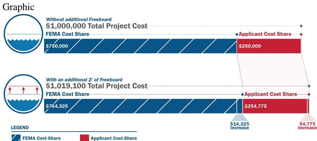
Freeboard: An additional amount of height above the Base Flood (1% annual chance) Elevation used as a factor of safety
