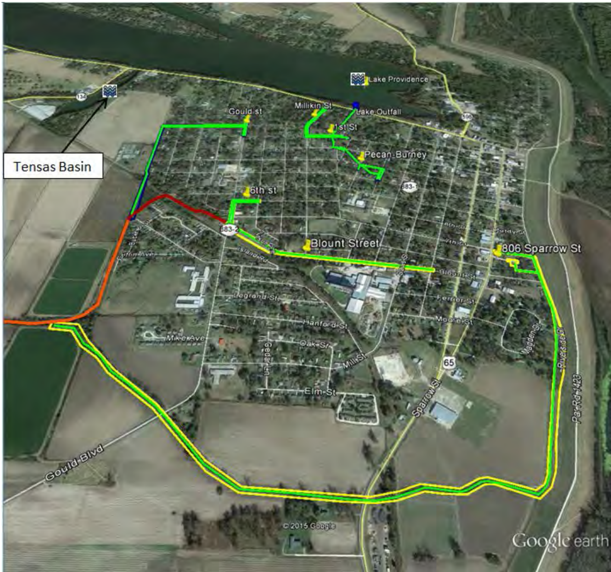
Figure 4: Drainage Improvements, Connection to Lake Providence Outfall
