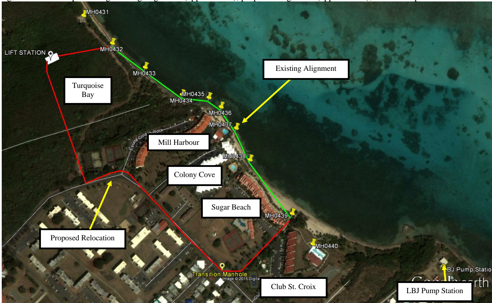
Figure 2. Aerial map showing existing alignment (approximate), proposed alignment (approximate), and development names.
