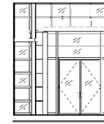
4 INTERIOR ELEVATION - LOBBY SOUTH A801 3/16" = 1'-0"
