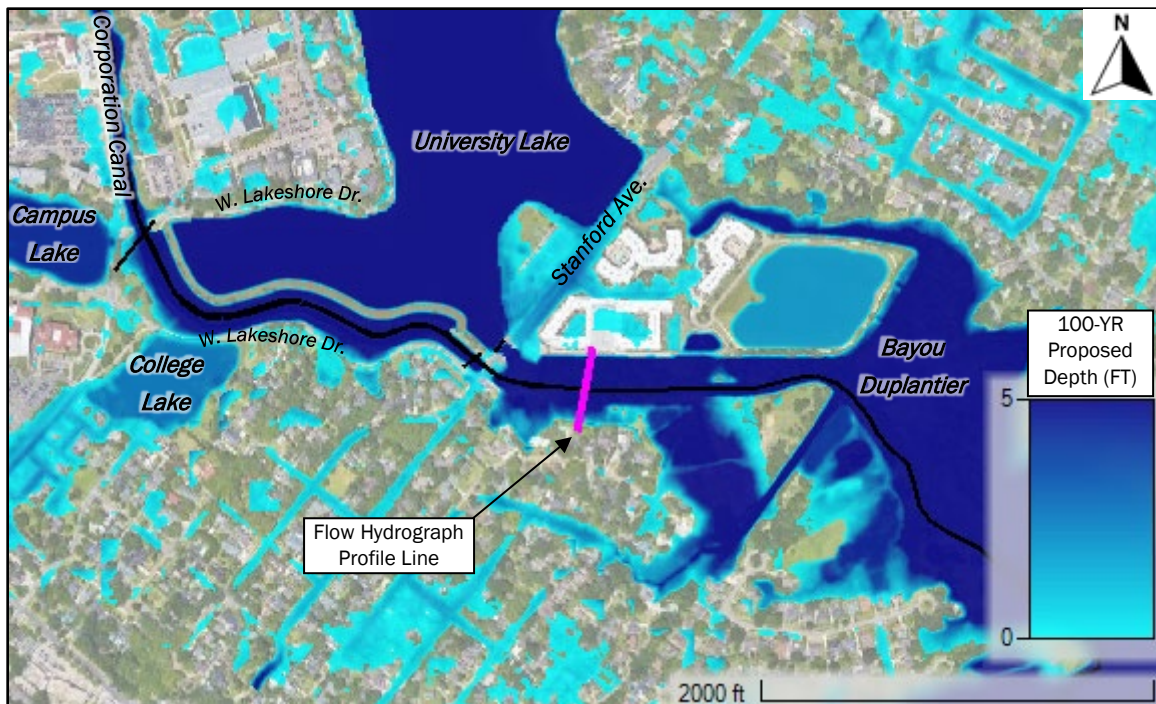
Figure 32: Bayou Duplantier Profile Line Location, Downstream of Stanford Ave.
