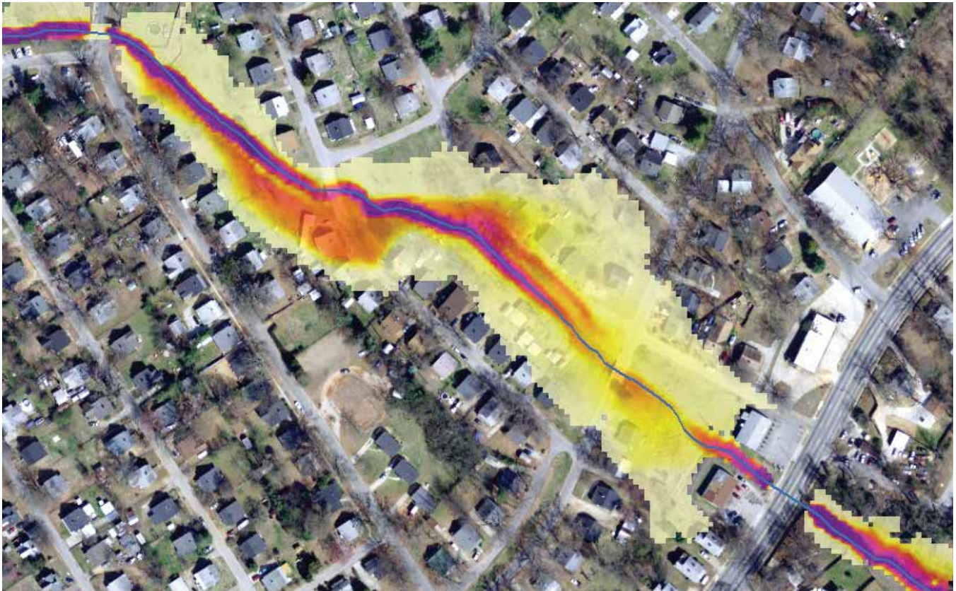
An enhanced non-regulatory dataset that can be provided as part of a Risk MAP project is a velocity grid or dataset. Velocity grids can provide valuable information for emergency responders and building science professionals
