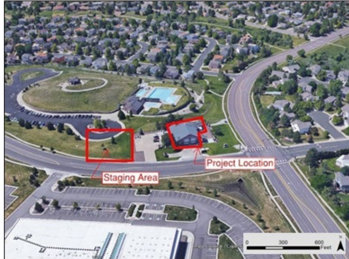
Figure 2. Example of a project site map. Map clearly shows the buildings to be retrofitted, the project area and the staging area. The map includes a north arrow and a scale.
