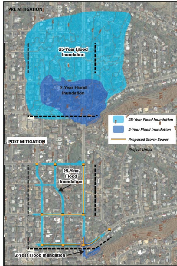
Figure 1. Example of before- and after-mitigation inundation map.
