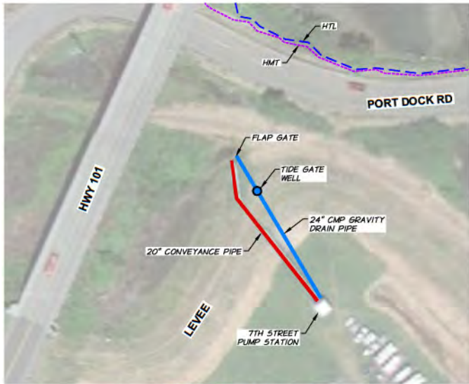
GRAVITY DRAIN NO. 5 TIDE GATE WELL
