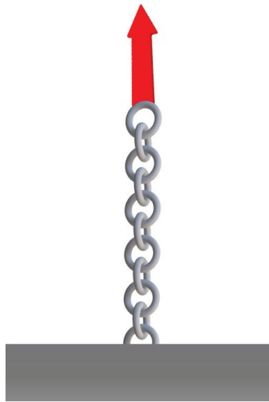
Figure 2-7 Chain illustrating the load path concept.
