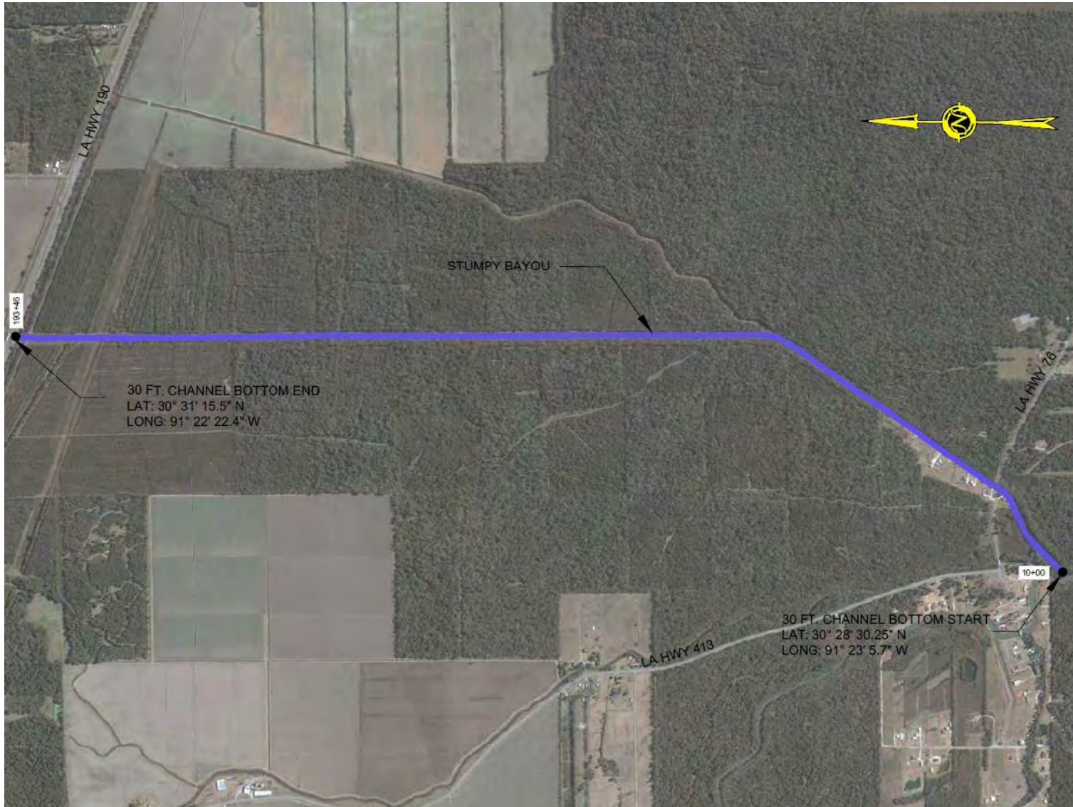
Figure 3. Plan View for the proposed 30 ft. channel bottom width segment of Bayou Stumpy for approximately 3.5 miles for the Bayou Stumpy Watershed Drainage Improvements Project provided by GIS Engineering, LLC.
