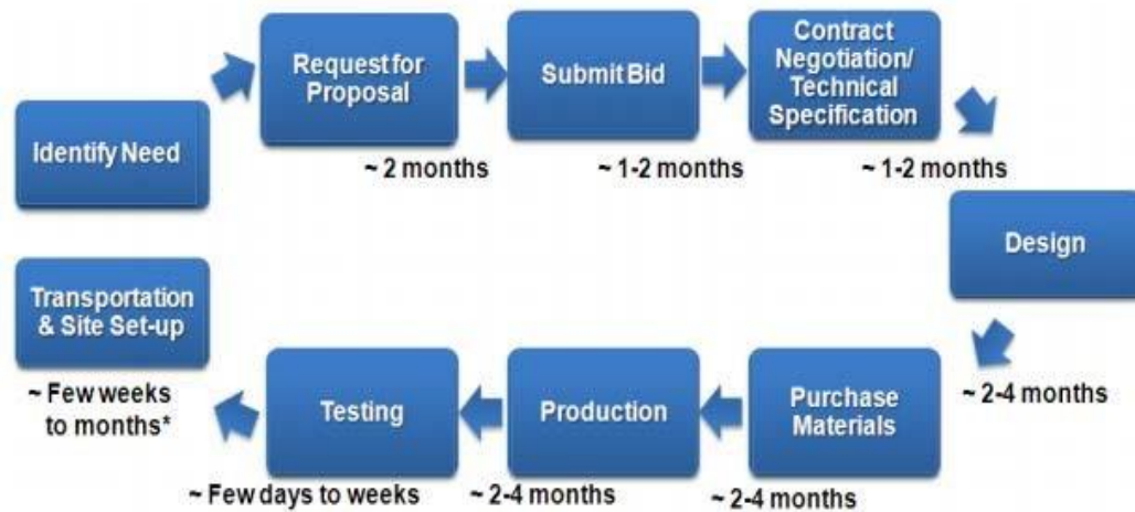
Figure 6: 2011 Large Power Transformer Procurement Process and Estimated Optimal Lead Time 21
