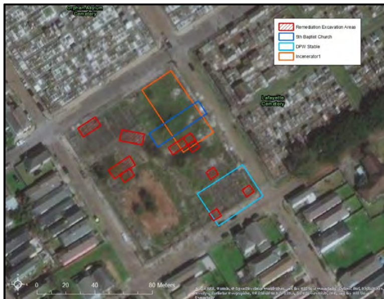
Figure 34. Current aerial photograph of the proposed Saratoga Stormwater Park (City Square 306) with areas to be remediated in red. Other colors are excerpts of building footprints from various Sanborn Fire Insurance maps.
