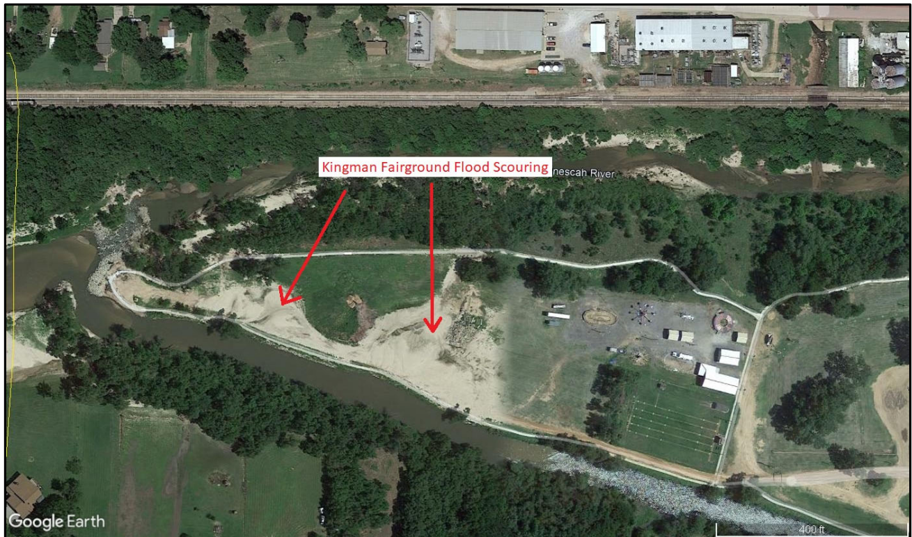
Figure 5. Aerial view of City of Kingman Parks – Kingman Fairgrounds Park (West Side) 2019 flood scouring
