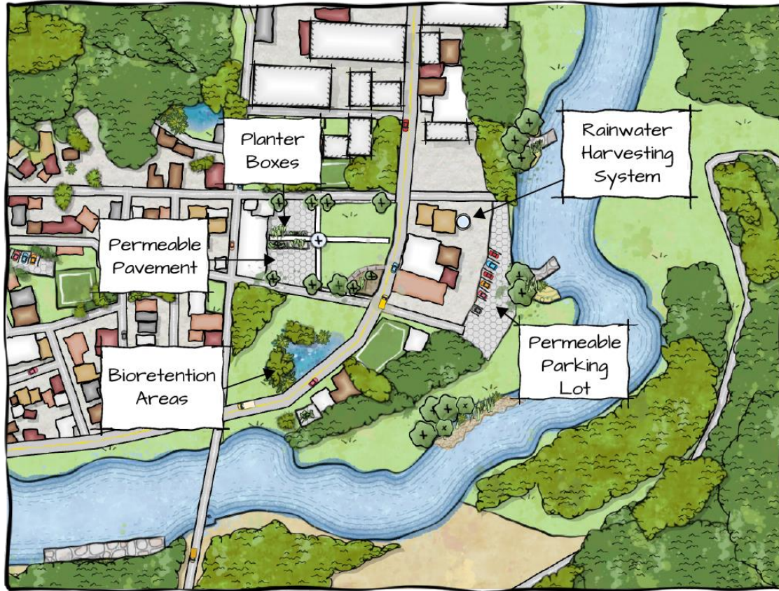
Figure 2-2: Example of how stormwater NNBS features can be incorporated into a community across various infrastructure types.
