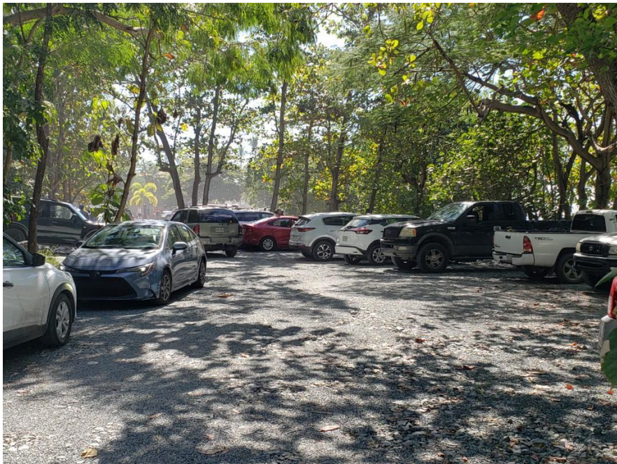
Figure 2-8. Permeable parking lot in Rincon, PR (Protectores de Cuencas, 2024)
