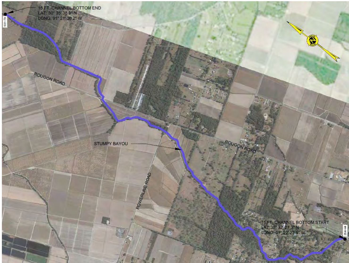
Figure 5. Plan View for the proposed 15 ft. channel bottom width segment of Bayou Stumpy for approximately 4.5 miles for the Bayou Stumpy Watershed Drainage Improvements Project provided by GIS Engineering, LLC.
