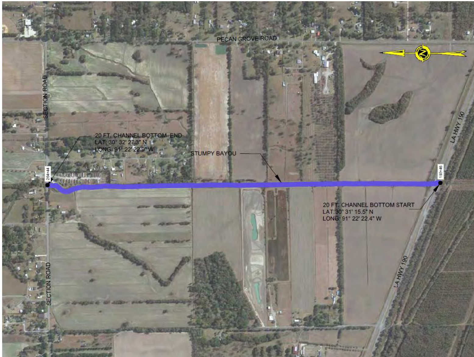
Figure 4. Plan View for the proposed 20 ft. channel bottom width segment of Bayou Stumpy for approximately 1.3 miles for the Bayou Stumpy Watershed Drainage Improvements Project provided by GIS Engineering, LLC.
