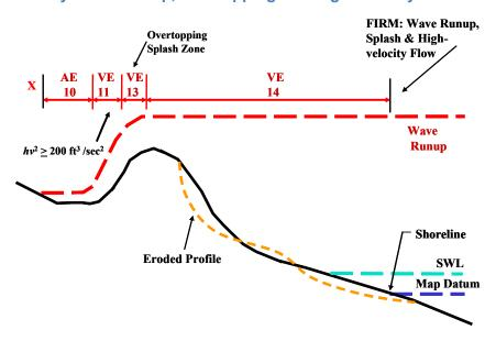
Figure 5-12. Cobble, Gravel, Shingle, or Mixed Grain Sized Beach with VE Zone Controlled by Wave Runup, Overtopping, and High-velocity Flow
