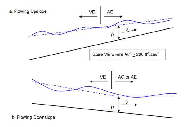
In the past there had been differing guidance on wave runup overtopping VE Zones and elevation determinations. In some areas it is standard practice to limit wave runup BFEs to 3 feet above the barrier crest when results show elevations higher than this. Additionally, a simplified runup procedure has been developed to delineate a VE Zone landward of the barrier when the potential runup is 3.0 feet or greater above the barrier crest, as shown in Figure 2-2.
