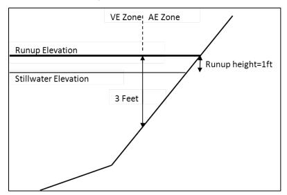
In general, the energy associated with the uprush of water from a broken wave (wave runup) is less than that associated with a breaking wave. Therefore, the runup height criterion should be equal to or greater than the 3-foot overland wave propagation wave height criterion. For consistency with other VE Zone criteria, and in the absence of data supporting a larger value, 3 feet was considered a reasonable value to use as the wave runup height criterion for mapping VE Zone.
