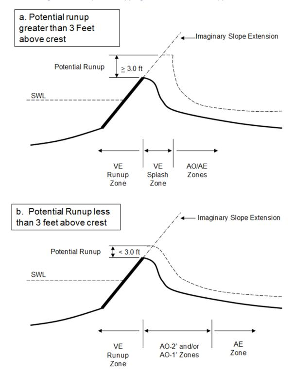
Figure 2-2. Simplified Mapping Procedure for Overtopped Barrier
