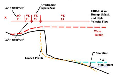
Figure 5-4. Erodible Low Coastal Bluff with VE Zone Controlled by Wave Runup,
