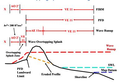
Figure 5-8. Sandy Beach Backed by Low Sand Dune with Overtopping Splash Controlling VE Zone
