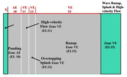
In this example, the potential runup is assumed to reach more than 3.0 feet above the crest, so an overtopping splash zone is mapped landward of the profile crest, with a high-velocity flow VE Zone and AE Zone to the rear. The AE Zone is mapped instead of the AO Zones shown in Examples 2, 4, and 5 because the overtopping ponds in the
