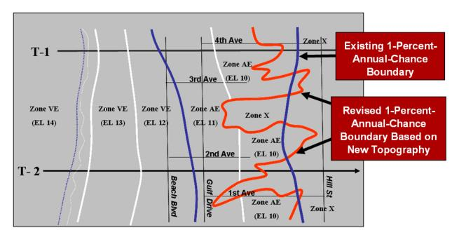
As shown in Figure 6-2, the redelineated limit of the 1-percent-annual-chance floodplain may impinge upon or cross flood zone boundaries located farther seaward. Similarly, a redelineated PFD limit may intersect flood zone boundaries located landward of the effective FIRM's PFD limit. The Mapping Partner shall not revise the location of gutter lines affected by the new 1-
