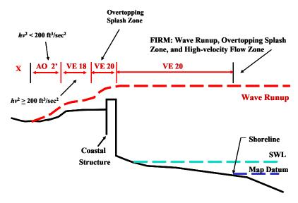
With shore structures having steep slopes, runup elevations are relatively high and a wide range of wave hazards can occur, including erosion or scour near the structure. These circumstances may result in a variety of distinct and compact situations, where appreciable engineering judgment can be required for appropriate assessment of flood hazards.
