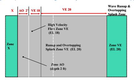
• **Example 6.** Figures 5-11 and 5-12 illustrate flood hazard mapping for a beach profile composed of gravel, cobble, or mixed grain sizes. In this example, the profile configuration should be determined in accordance with <u>Coastal Erosion Guidance</u>, and the wave hazards should be modeled using the eroded profile. There will be no PFD designation for a gravel, cobble, or mixed grain size profile, so the mapped hazard zones and BFEs will reflect calculated flood hazards only.
