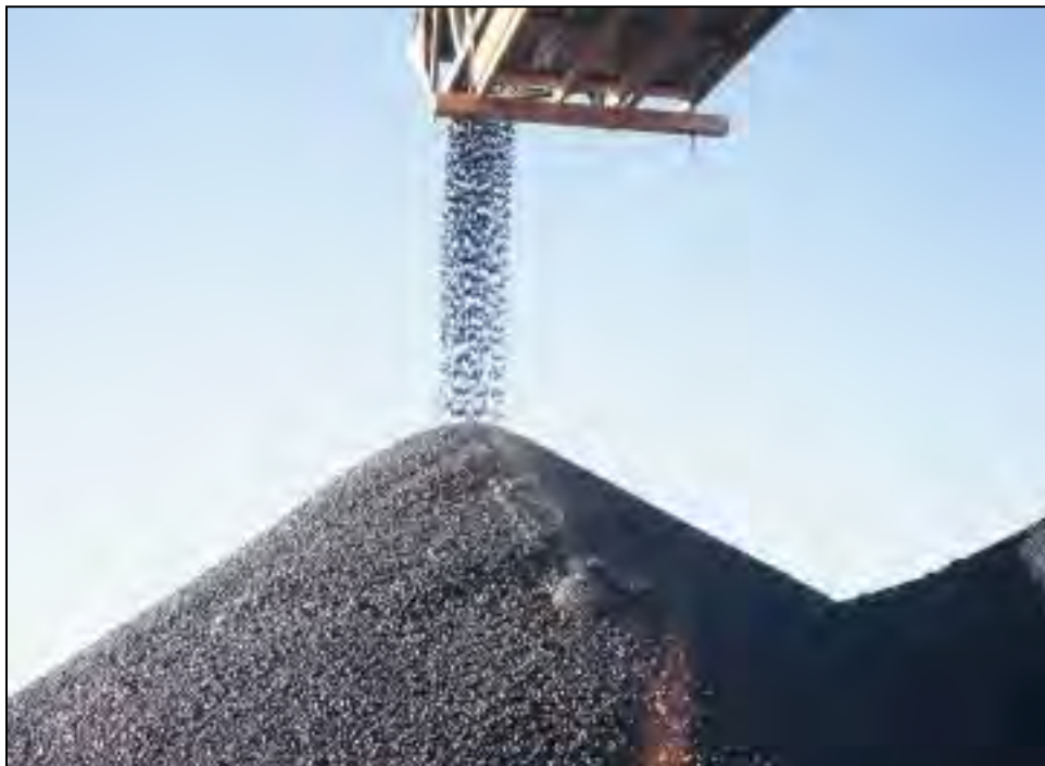
Figure 7-10. High drop height at belt discharge.
