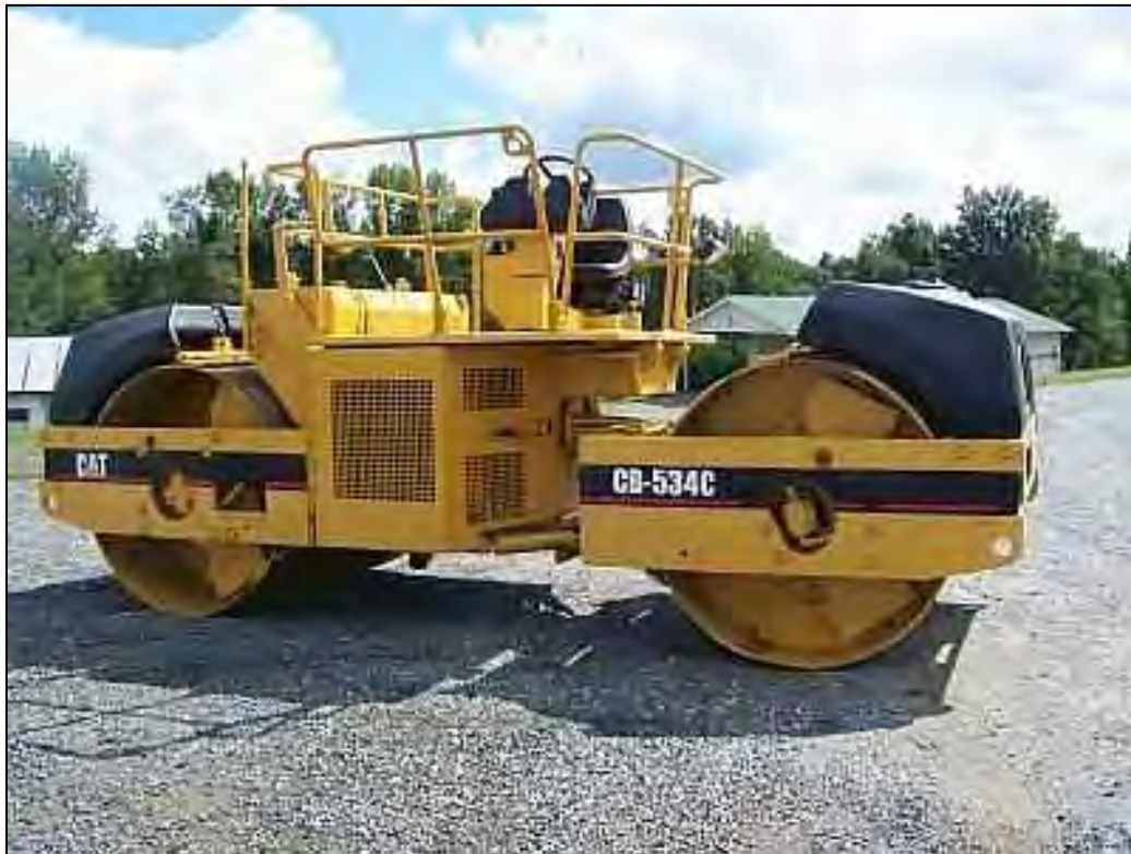
Figure 7-21. Double-drum vibratory roller.
