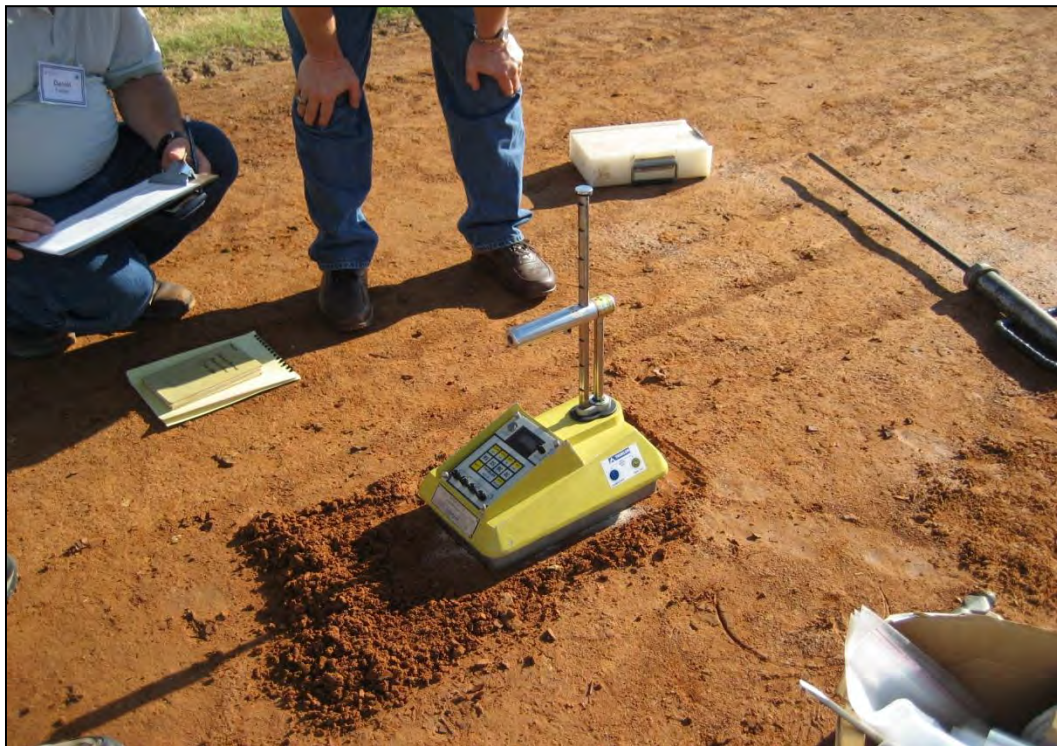
Figure 7-29. Typical nuclear moisture-density meter.
