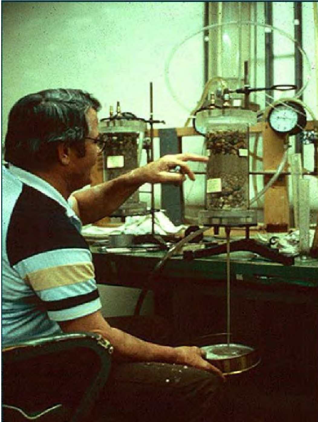
Figure F-3. No erosion filter testing being conducted in Soil Conservation Service laboratory in Lincoln, Nebraska. (Photo credit - James Talbot.)
