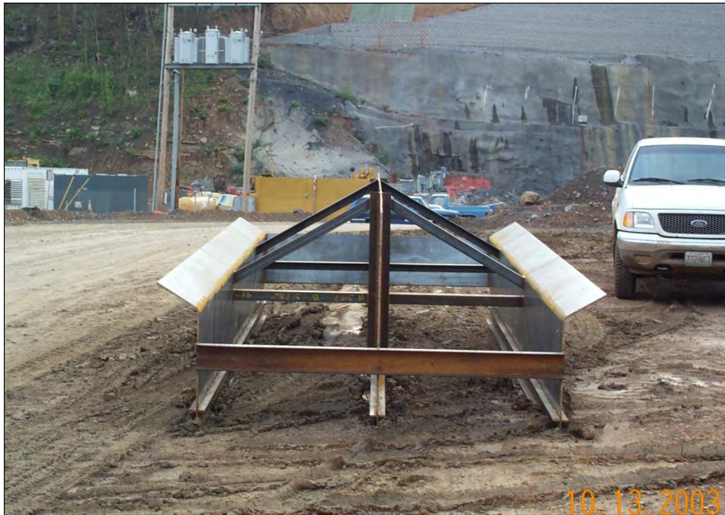
Figure 7-15. Double-bin spreader box.
