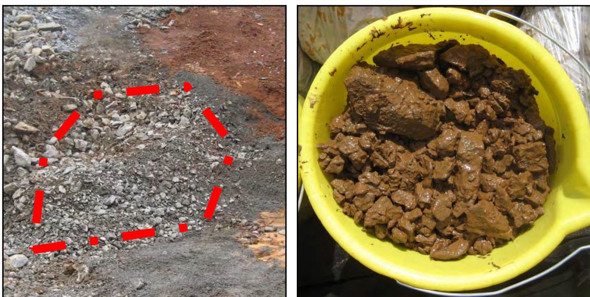
Figure E-13. Comparison between normal gray medium filter (left) and medium filter contaminated with red-brown clay from near the missing fine filter.
