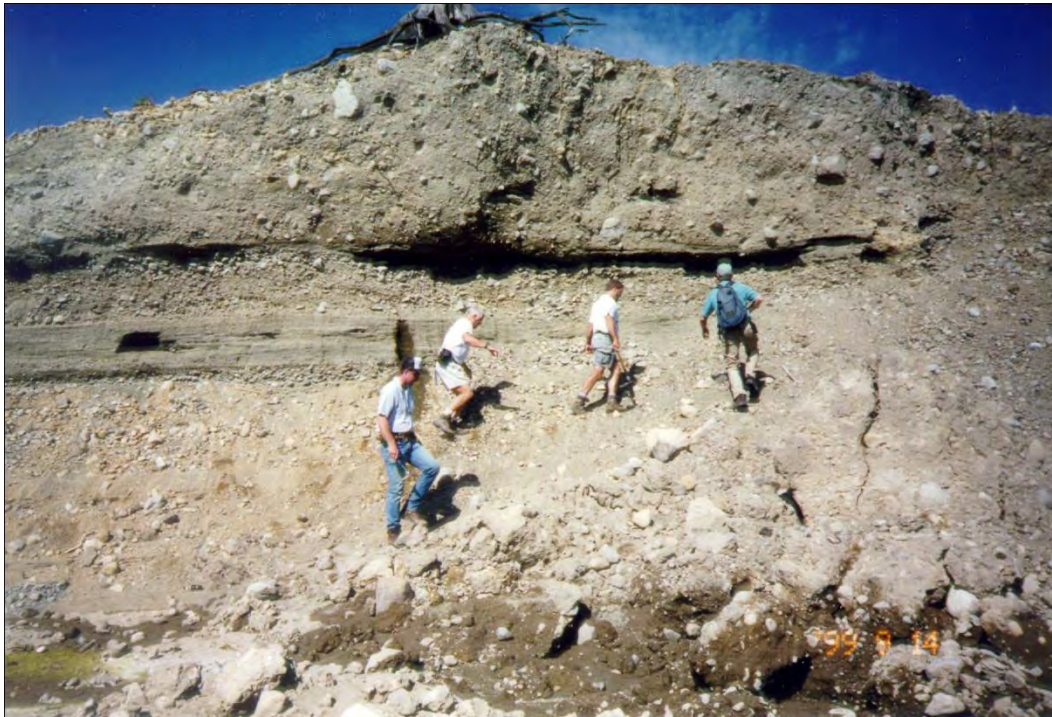
Figure 6-7. Exposed moraine cross section showing till overlying glacial outwash. Such exposures provide an opportunity to obtain geologic information without an expensive exploration program.
