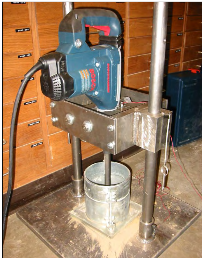
Figure 7-31. Vibratory hammer used to obtain a reference density value for filter materials. (Photo courtesy of Dr. Vincent Drnevich)
