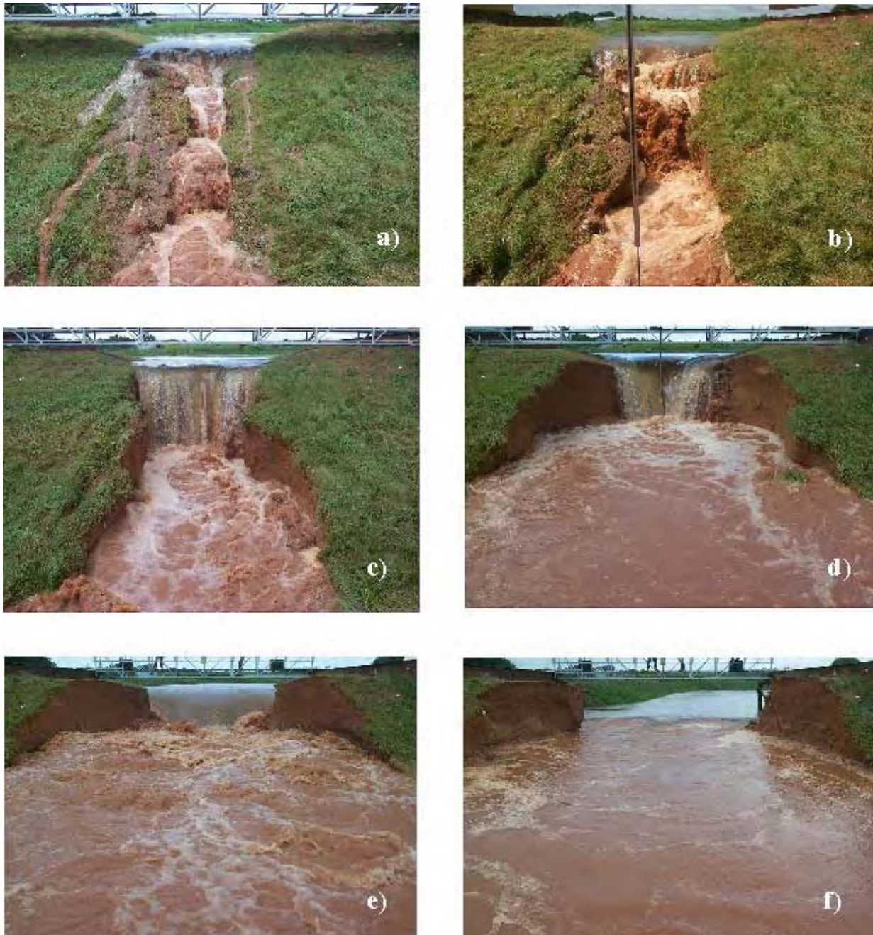
Figure 12. Generalized description of observed erosion processes during ARS overtopping tests: a) rills and cascade of small overfalls during Stage I, b) consolidation of small overfalls during Stage I, c) headcut at downstream crest, transition from Stage I to Stage II, d) headcut at upstream crest, transition from Stage II to Stage III at breach initiation t = t_i , e) flow through breach during Stage III, and f) transition from Stage III to Stage IV at breach formation t = t_f .
