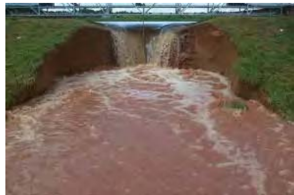
d) Headcut at upstream crest, transition from Stage II to Stage III at t = t_2 = 31 min, t_i .
