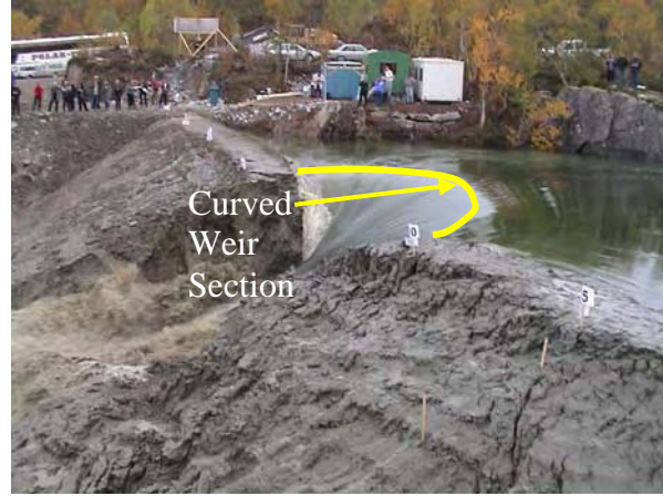
Figure 14. Curved weir control section during breach formation during Norway test.
