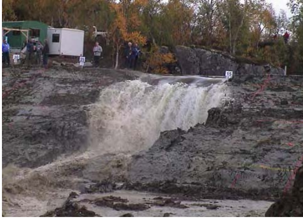
Figure 13. Observed headcut erosion during cohesive embankment overtopping test in Norway
