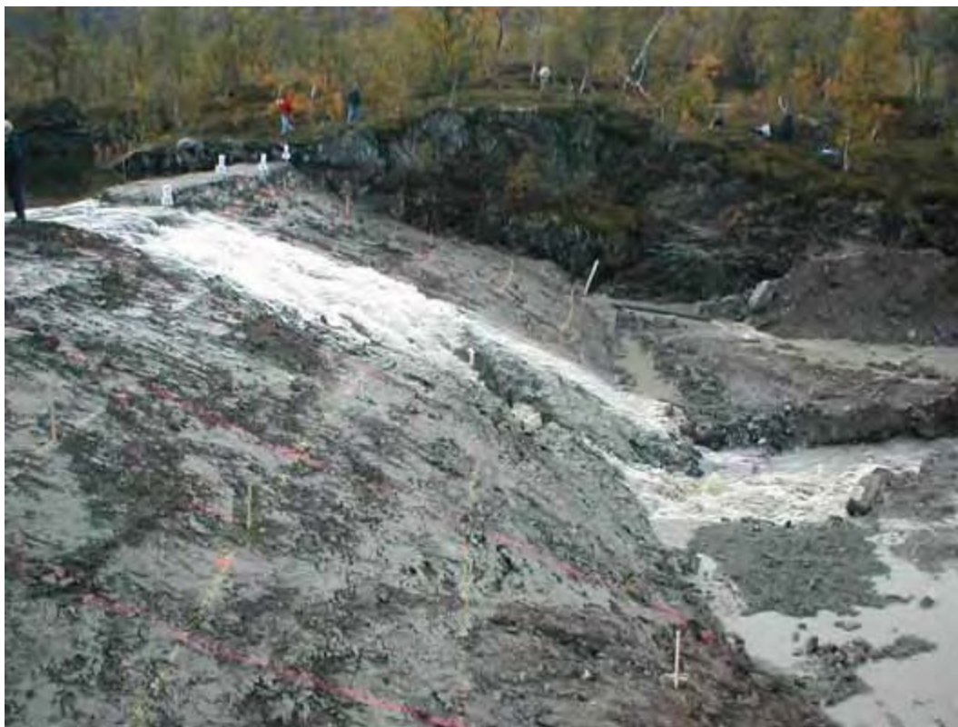
Figure 17. Beginning of erosion at the toe of the embankment as headcuts are formed.
