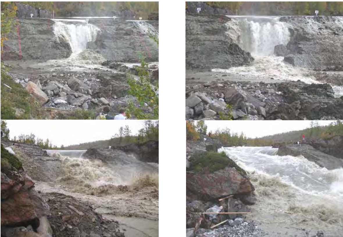
Figure 6 Pictures taken during the test of the clay dam
