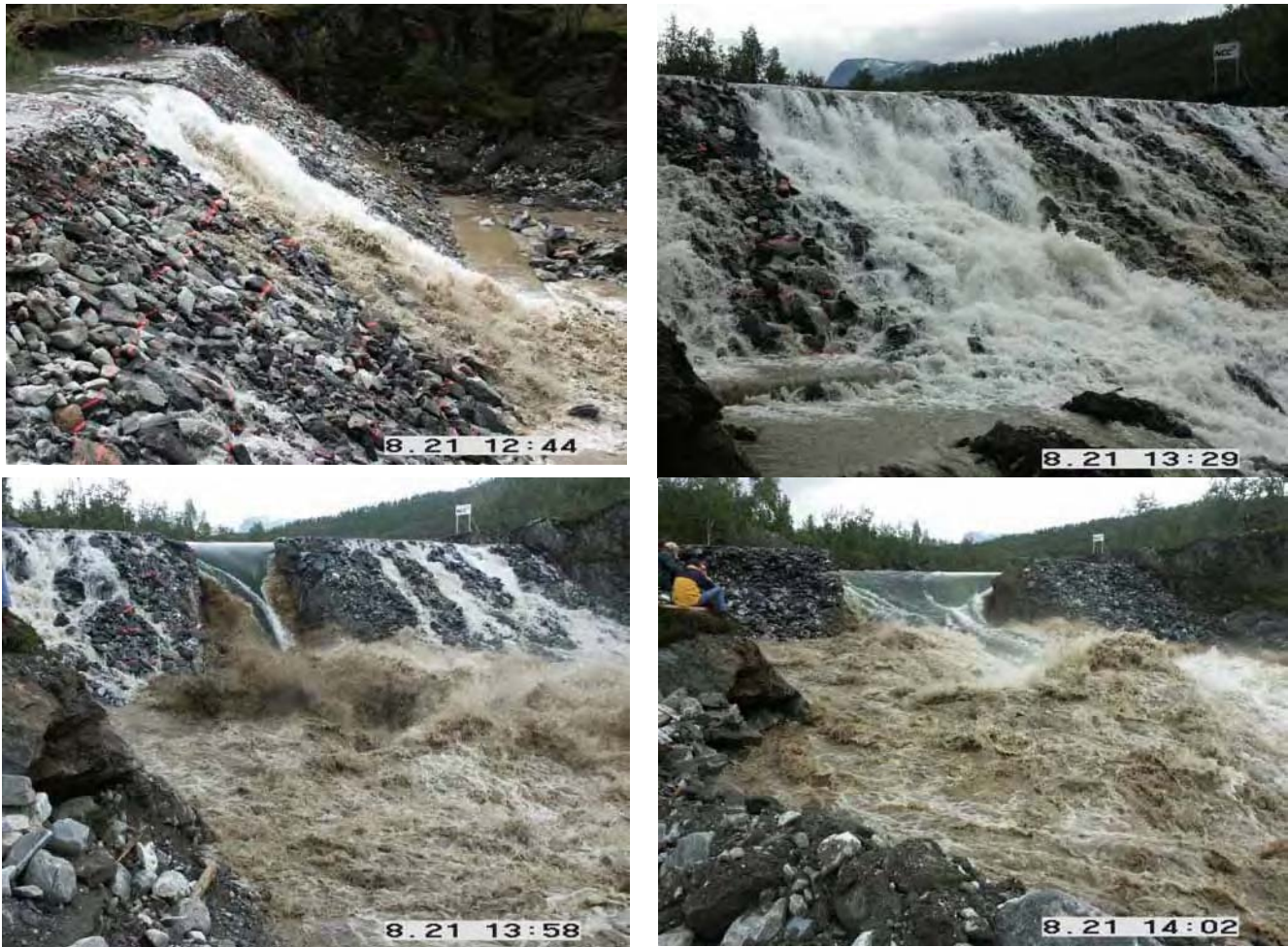
Figure 13 Pictures from test with rockfill dam with moraine core.
