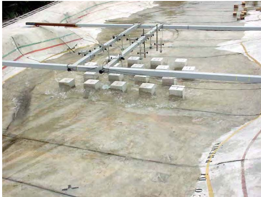
Figure 7: A model city flooding test run.
