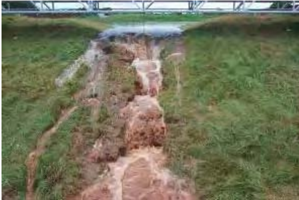
a) Rills and cascade of small overfalls during Stage I at t = 7 min.
