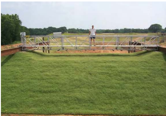
Figure 9. Embankment overtopping setup at ARS Hydraulic Laboratory
