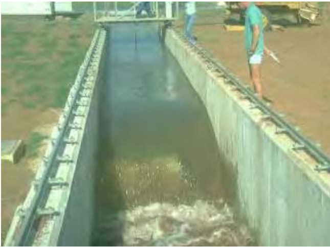
Figure 3. Headcut migration test in large outdoor flume.
