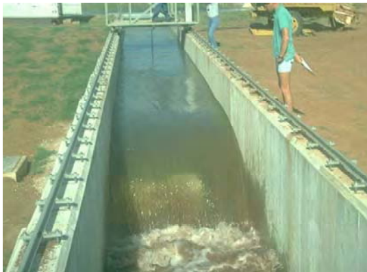
Figure 7. Headcut migration test in large outdoor flume.
