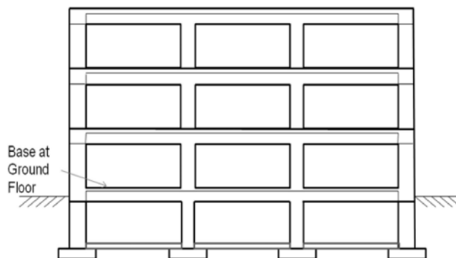
FIGURE C11-3 Base at Ground Floor Level
