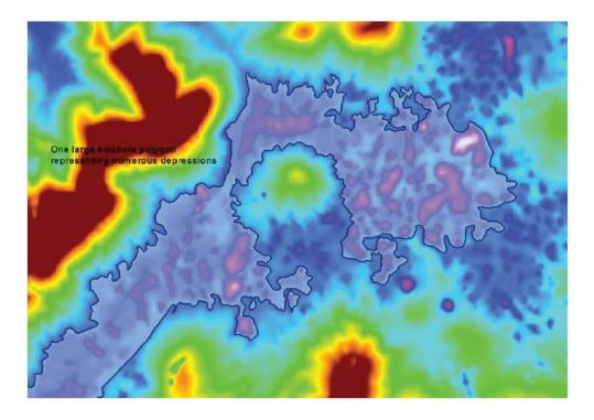
Figure 1: Large Sinkhole Polygon Representing Numerous Depressions
