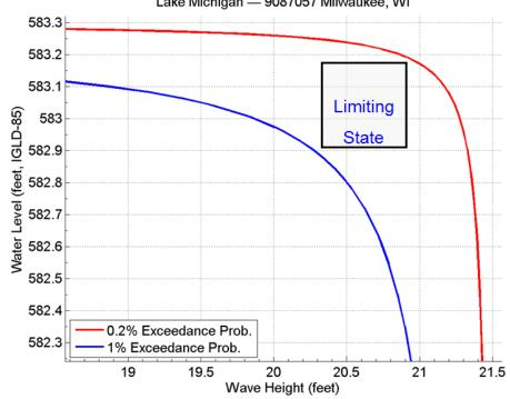
In deepwater,  $H_{m0}$  is approximately the same as significant wave height  $(H_s)$ , but in shallow water,  $H_{m0}$  is 10 to 15 percent smaller than the  $H_s$ . This difference in wave height definition must be accounted for where necessary.
