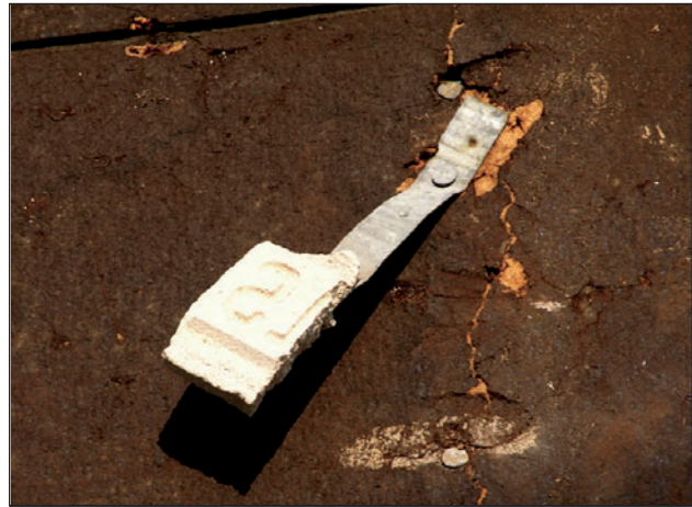
Figure 6. This tie was embedded in the mortar, but the bond was poor.
