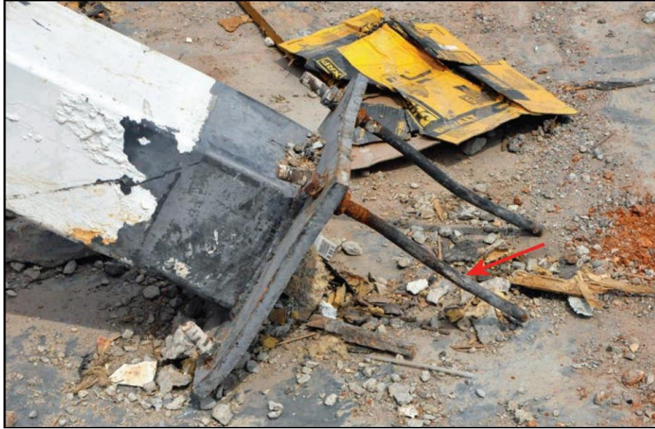
Figure B3-9: Bolt failure at interior column resulting from shear and tension. The hooked anchor bolts pulled out of the slab (red arrow) (Joplin, Missouri 2011 tornado)
