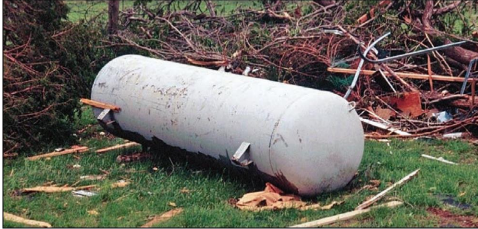
Figure B8-6: Large debris: Propane tank that was blown from its original location (Midwest tornadoes, 2007)
