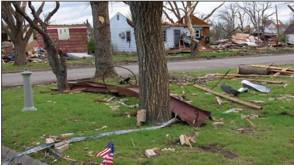
Figure B8-15: Steel beam debris (Greensburg, Kansas, 2007 tornado)
