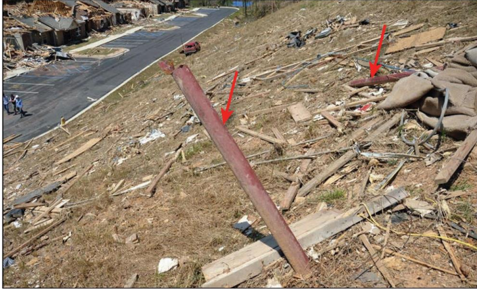
Figure B8-14: Steel porch column debris from an apartment complex where columns that were 7 feet 9 inches long and 4¼ inches in diameter (see red arrows) had a significant upward trajectory and flew approximately 230 feet (Tuscaloosa, Alabama, 2011 tornado)
