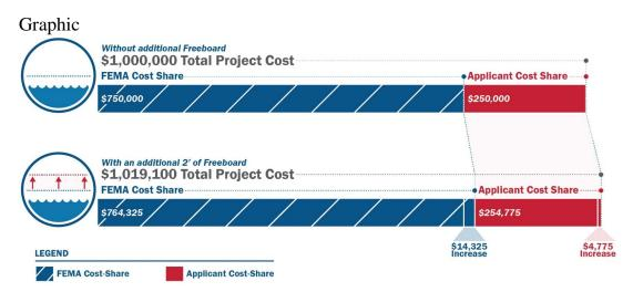
Freeboard: An additional amount of height above the Base Flood (1% annual chance) Elevation used as a factor of safety
