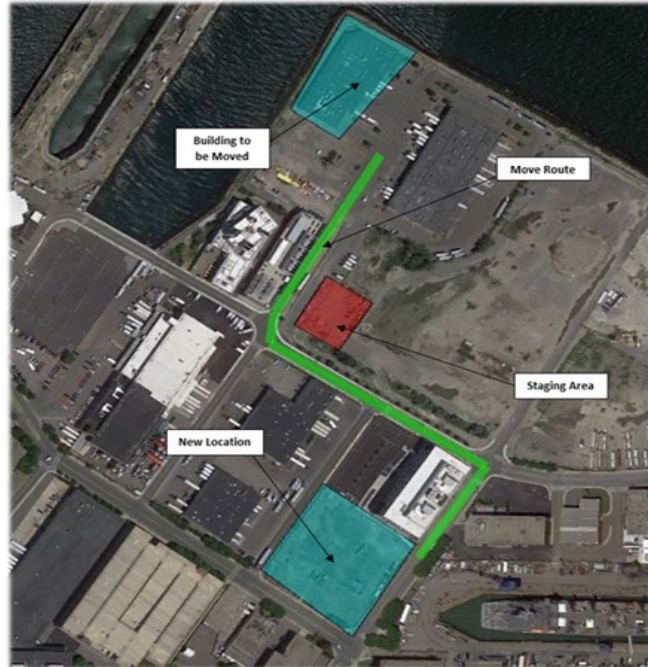
Figure 2. Example of a project site map. Map clearly shows the locations of the existing building and the new location where it will be moved to, the staging area and the access route between the two locations. The site features are overlaid on an aerial photo.
